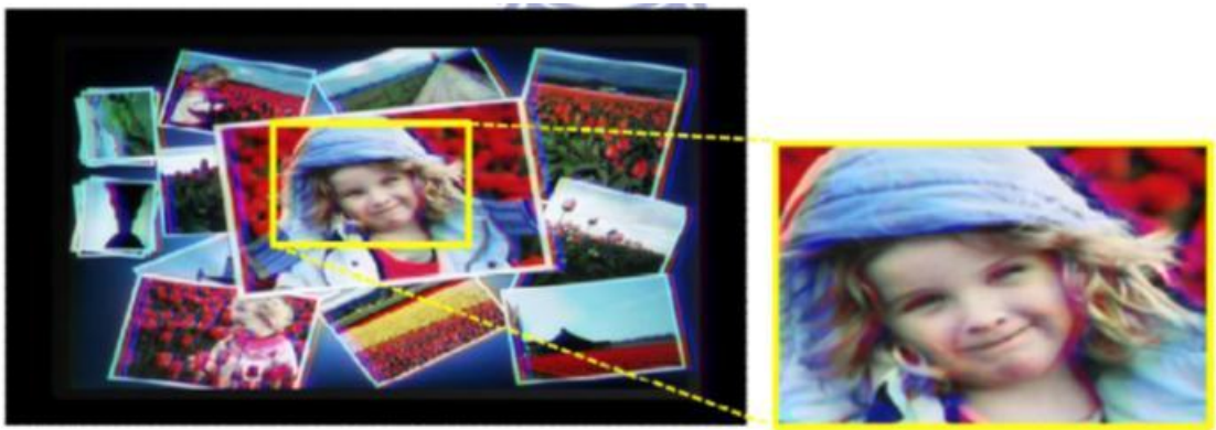
(c) Color breakup image of the 180Hz Stencil-FSC method with target image Girl
