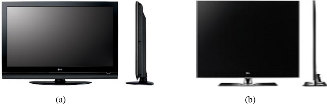
Fig. 1-8 Two backlight types of LCDs: (a) direct-lit backlight, and (b) side-lit backlight.
