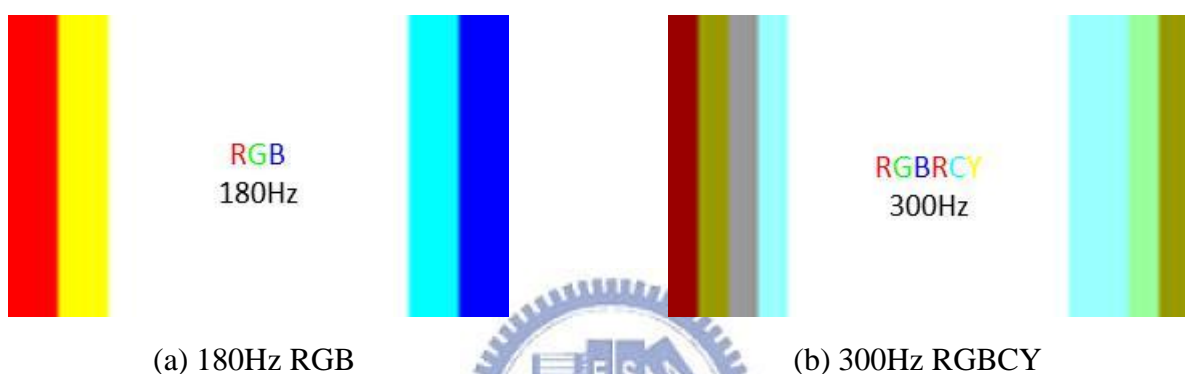
Fig. 2-10 Simulation color breakup image of (a) 180Hz RGB, and (b) 300Hz RGBCY.
