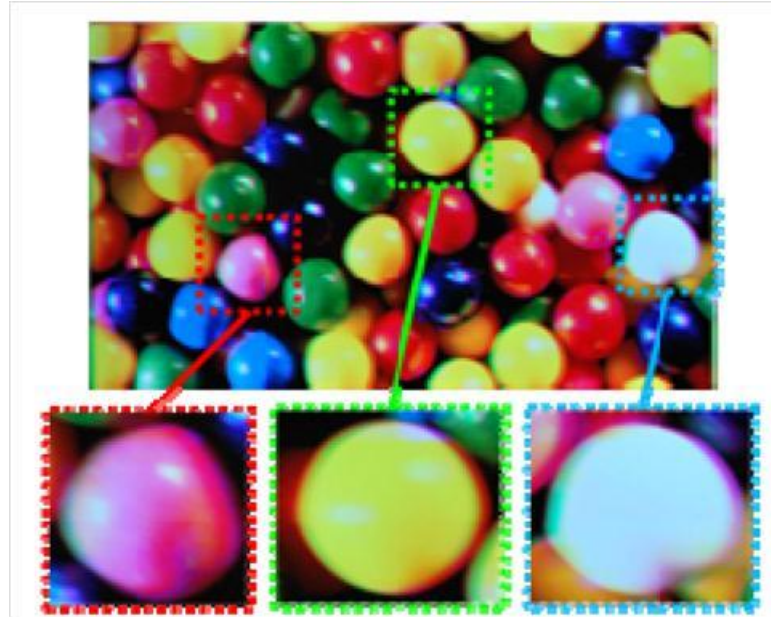
(a) Color breakup image of two-color-field method with target image Color Ball
