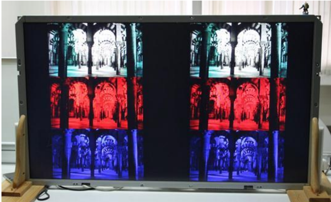
Fig. 4-10 The 46-inch 120Hz MVA LCD for verifying color breakup phenomenon.
