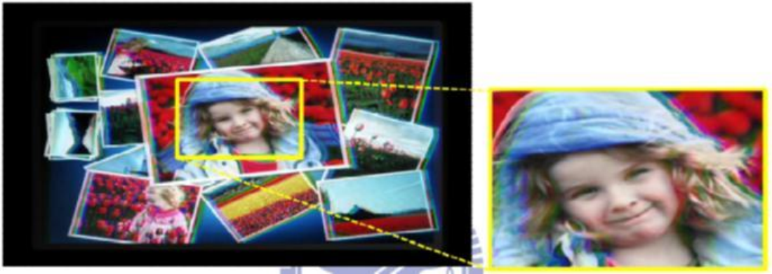
(b) Color breakup image of 240Hz Stencil-FSC method with target image Girl
