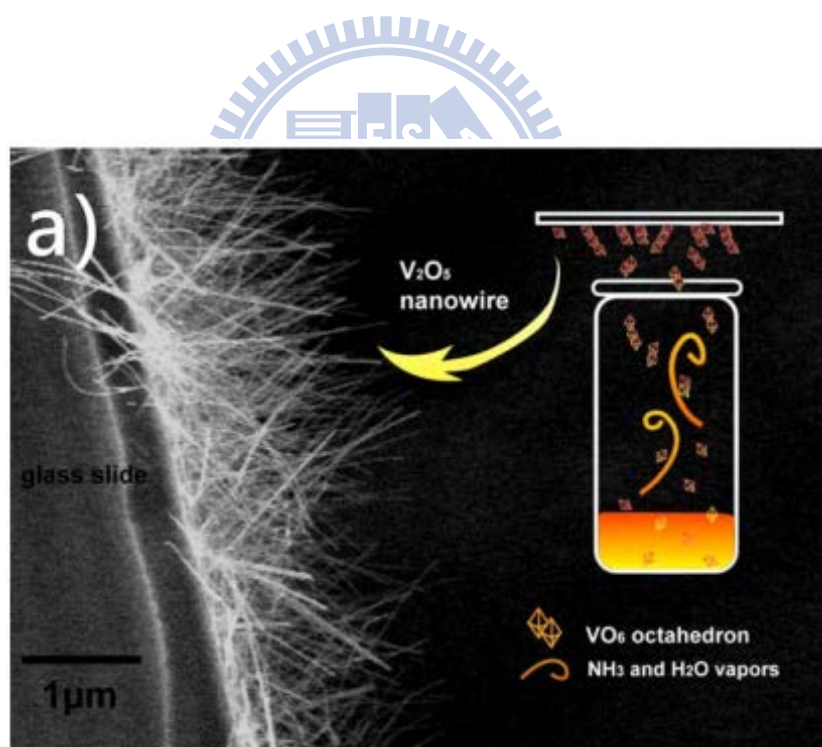
Figure 1.9 Schematic illustration of experiments to deposit V_2O_5 NWs on the surface of a substrate. 62
