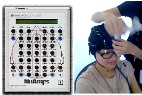
Figure 1.1: EEG measuring devices. From left to right is the EEG amplifier and the electrode cap.
