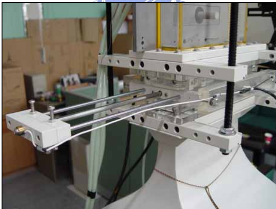
Fig. 2.18 The structural configuration of smoke generation
