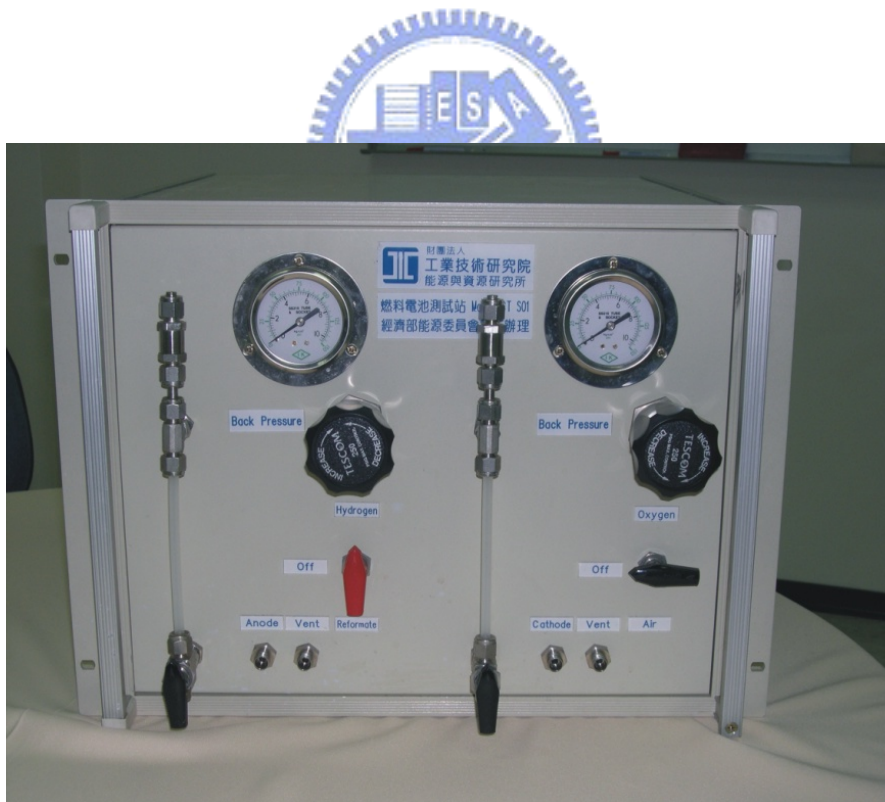
Fig. 2.5 The gas pipelines controller
