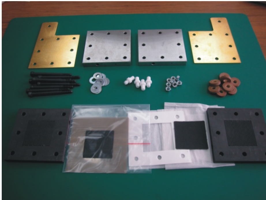
Fig. 2.11 All components of PEMFC
