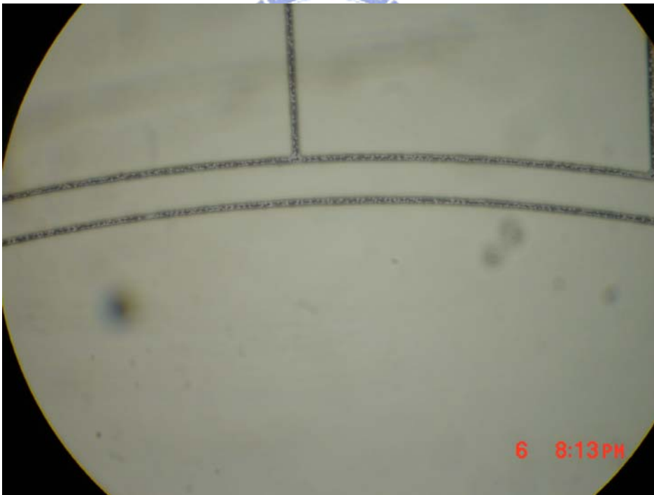
Fig. 3.4 After etching aluminum process.
