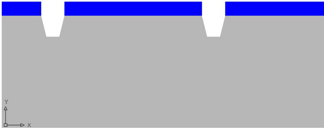
Fig. 4.5 The profile of the SiO 2 mask.
