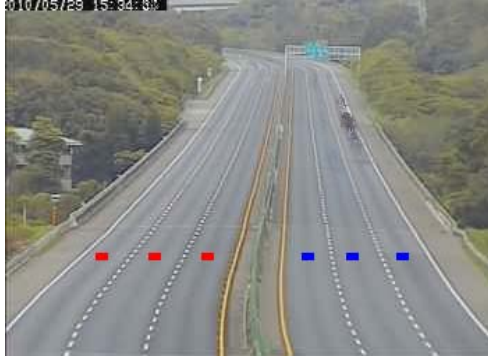
Figure 11. Results of virtual detectors installation on a bidirectional roadway.
