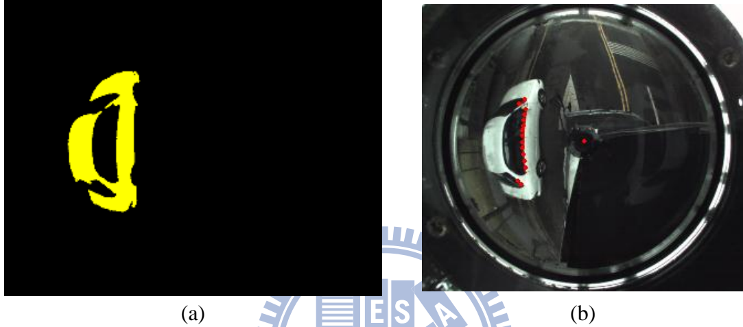
Figure 5.7 An example of edge-point extraction. (a) The bi-level image b for searching the bottom-edge points of the vehicle window (a) An image to show the result of finding the edge points, and the red points represent the edge points corresponding to (a).
