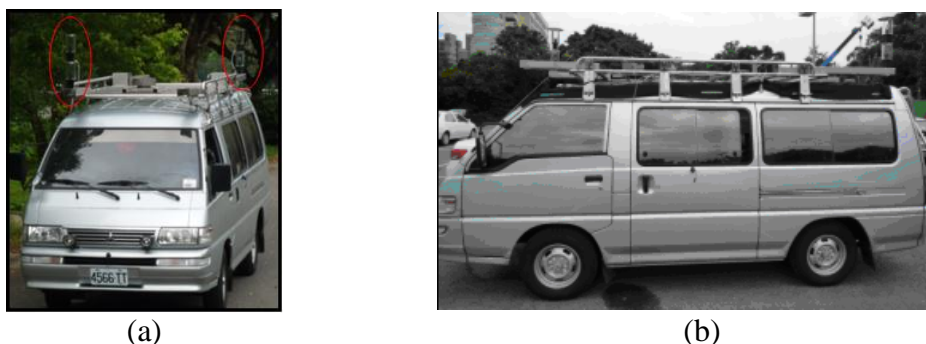
Figure 2.1 The video surveillance vehicle used in this study with a pair of two-camera omni-directional devices affixed on the car roof. (a) A front view of the video surveillance vehicle. (b) A side view of the video surveillance vehicle.
