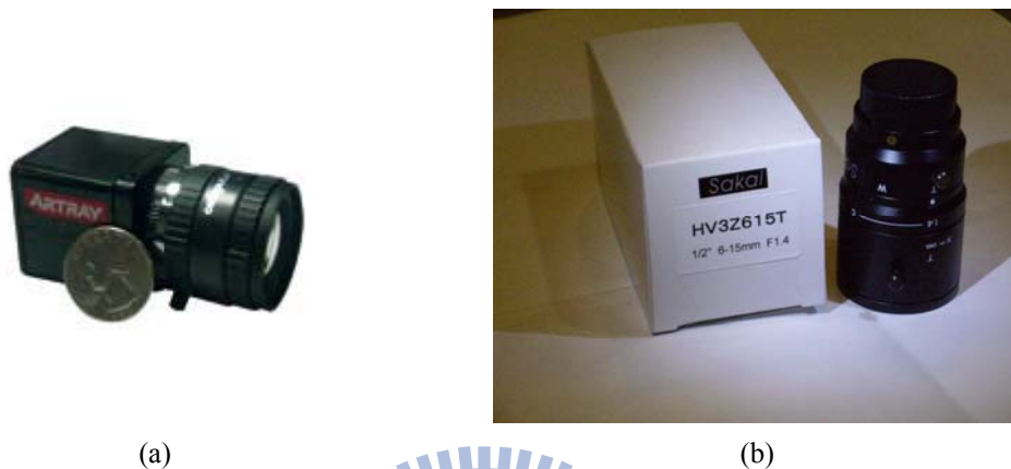
Figure. 2.4 The used camera and lens. (a) The camera of model Arcam 200so produced by ARTRAY Co. (b) The lens produced by Sakai Co.
