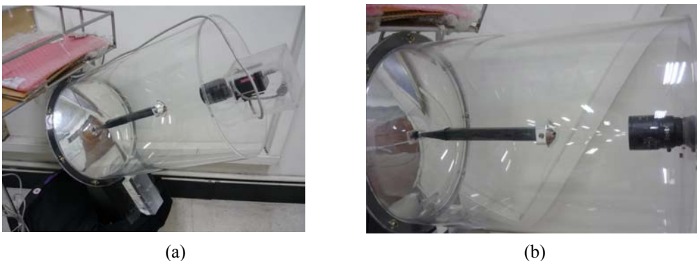
Figure. 2.3 The two-mirror omni-camera used in this study. (a) A full view of the camera equipped on the vehicle. (b) A closer view.
