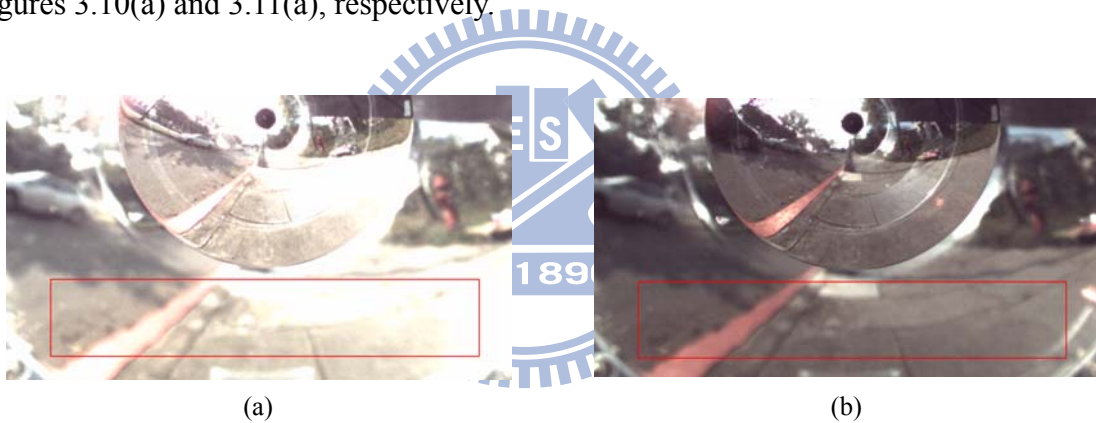
Figure 3.9 Two different illuminations in the image for curb detection and the environment windows. (a) An instance of overexposure. (B) A suitable case.
