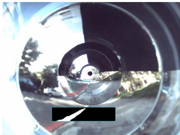
Figure 7.6 Image of a result of curb line detection.
