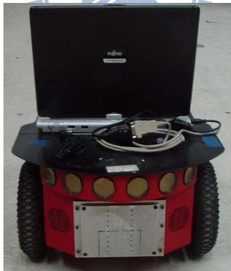
Figure. 2.1 Autonomous vehicle, Pioneer 3 produced by MobileRobots Inc., used in this study.
