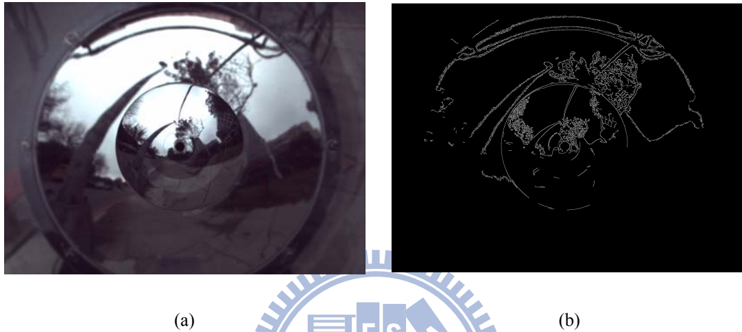
Figure 5.7 Two omni-images with the projection of the light pole. (a) The input image. (b) The result edge image after doing Canny edge detection.
