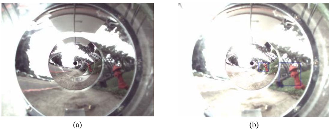
Figure 3.10 Two different illuminations in the image for hydrant detection and the environment windows. (a) An unclear case. (B) An appropriate case.
