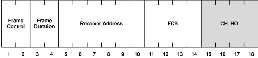
Figure 2.8: Frame Format of the control packet GRANT_{CR}
