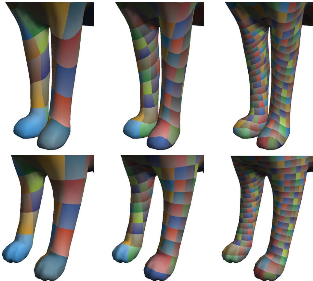
Figure 4.13: The cross-parameterization of the front legs between the lion (top) and cat (bottom). The texture repeat cycle is doubled from left to right to clarify the result.
