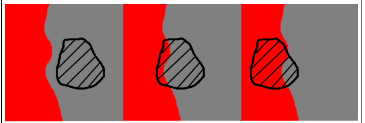
Figure 3: Handling the occlusion parts of the disparity maps. Red area is occlusion parts and grey area is known disparity values. Black slash area is one of the segments. Left, middle and right picture shows the segment of \tilde{S}_{Non\_Occ} , \tilde{S}_{Part\_Occ} and \tilde{S}_{Occ} .
