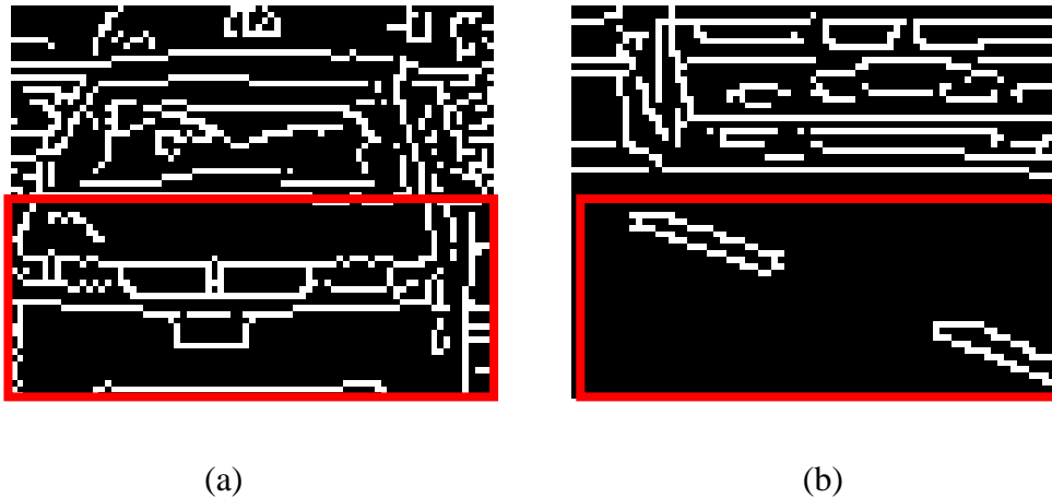
Figure 3-12 Example of bottom-half part of (a) vehicle and (b) non-vehicle
