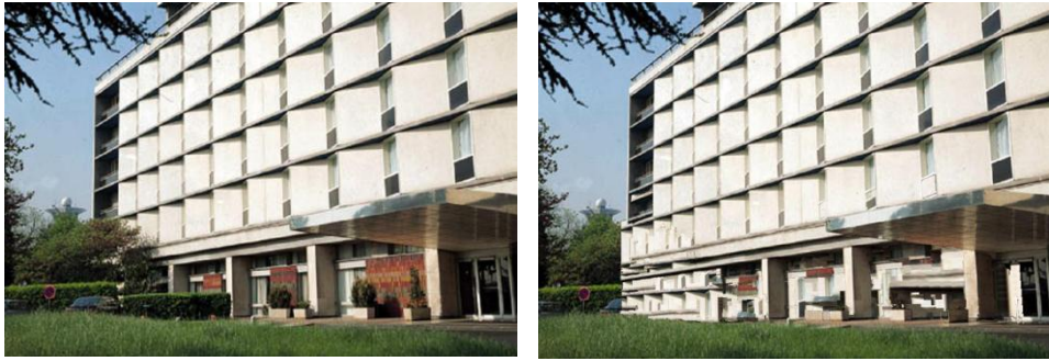
Figure 5.4 Left is the origin input image , right is the perspective inpainting results for foreground obstacle removal.
