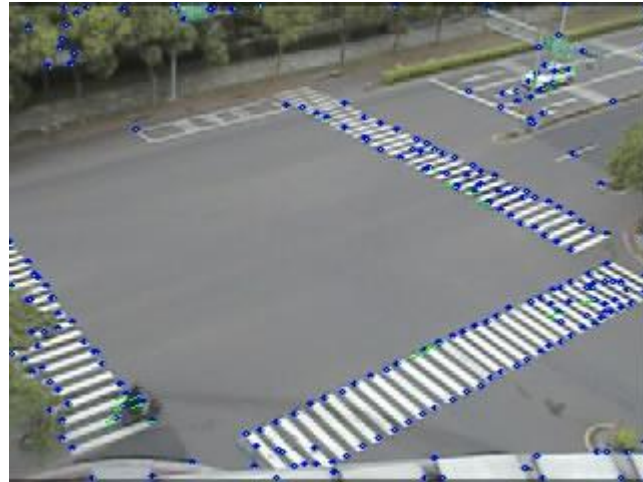
Figure 12 The blue point is the guess feature points of frame no.2. The green line is the results of KLT algorithm
