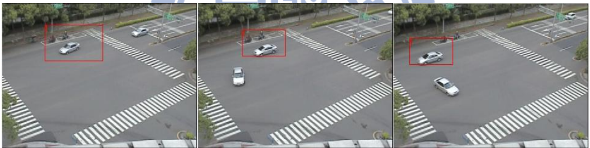
Figure 35 Experimental results of object tracking by Mean-shift
