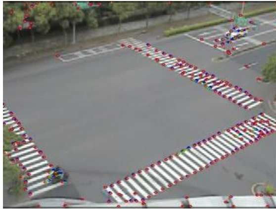
Figure 15 Video frame after KLT algorithm
