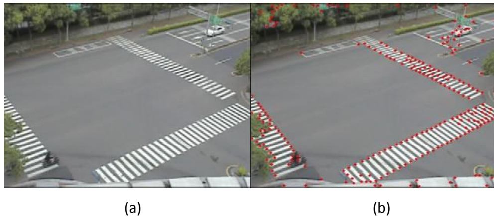
Figure 10 (a) Input original frame (b) KLT corner detector of original frame
