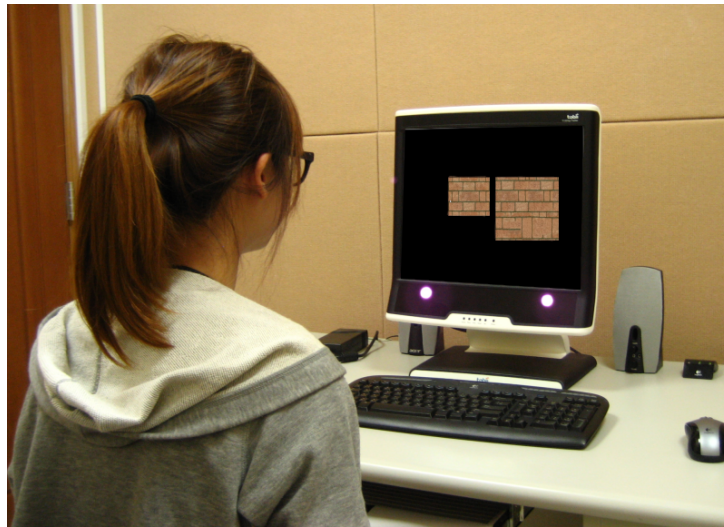
Figure 3.1: This photo shows Tobii T120 Eye-tracker and experiment environment.
