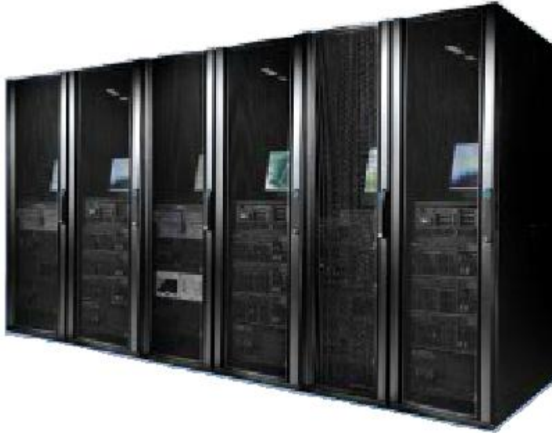
Figure 3.1 The picture of a IP-based lock and rack server enclosure
