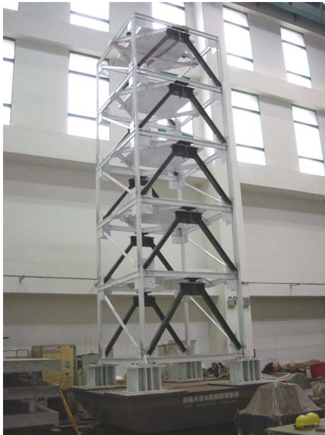
Fig. 5.4 Seismic performance test of the damper on a model structure via shaking table
