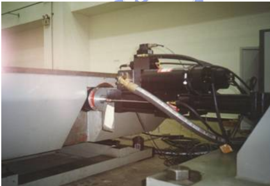
Fig. 5.3 15-ton dynamic actuator of MTS
