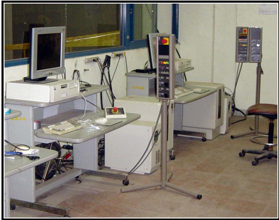
Fig. 4.18 MTS control system in the control room
