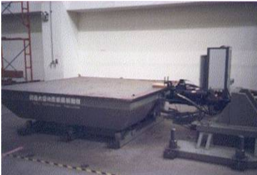
Fig. 5.2 Earthquake simulator -- shaking table system
