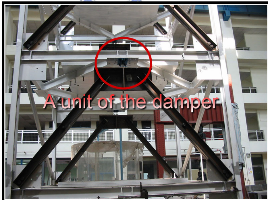
Fig. 5.5 A close-up view of a unit of the damper on the model structure
