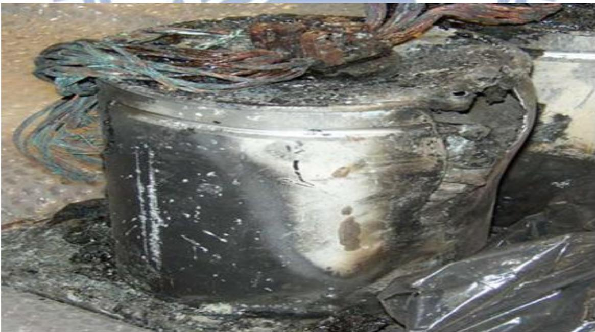
圖 7: Burst pressure vessel of a line filter capacitor (Image source: Allianz)
