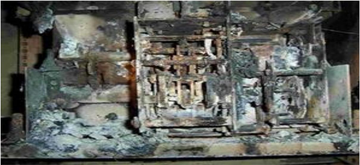
圖 6: Power switch of a 1 MW wind turbine - destroyed by fire (Image source: Allianz)
