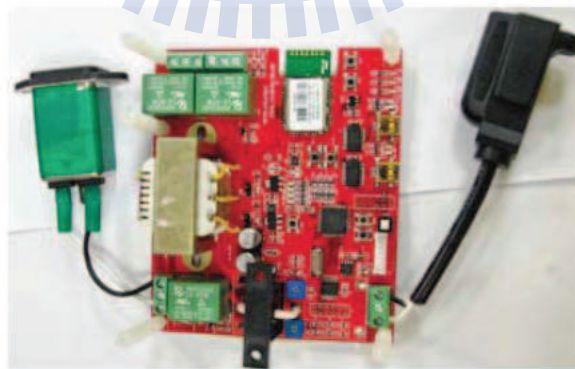
Figure 4.2: Our implemented wireless power meter.
