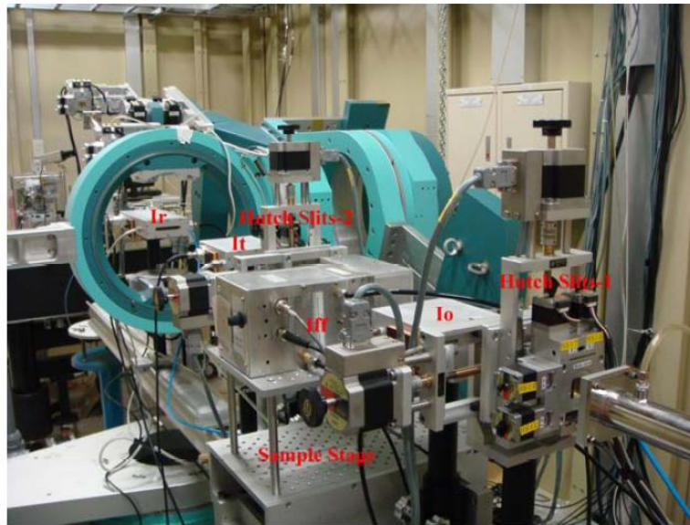
Fig. 2-1: The instruments used in BL07A. The I_0 in the photo is the ion chamber used to estimate photon flux. The sample stage is where we put the devices on.
