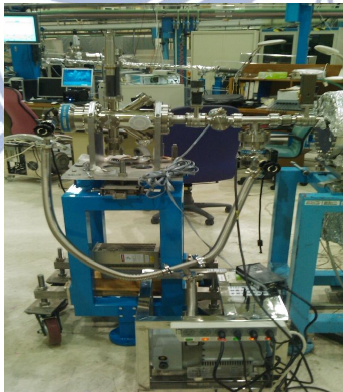
Fig. 2-2: End station in BL08A, including main chamber, two turbo pump and a mechanical pump.
