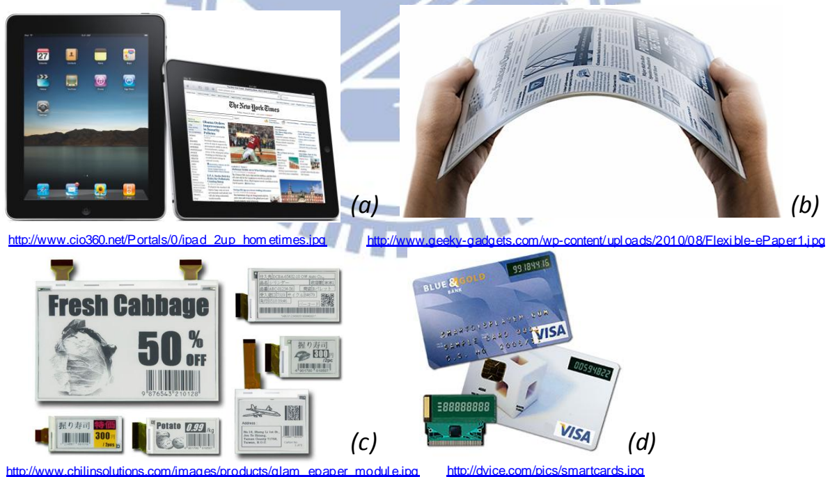
Fig. 1-1 E-paper products (a) E-books. (b) Flexible displays. (c) Price tags. (d) Smart cards.
