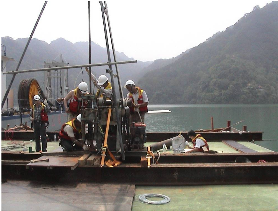
Fig. 6-5 Operation of TDR/DMT from a barge
