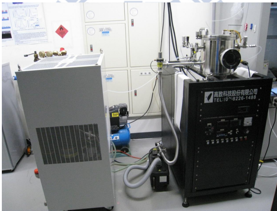
Figure 2-2 6 The annealing system is used in the bonding process.
