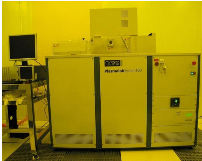
Figure 2-2 8 The ICP-RIE system is used for dry etching.
