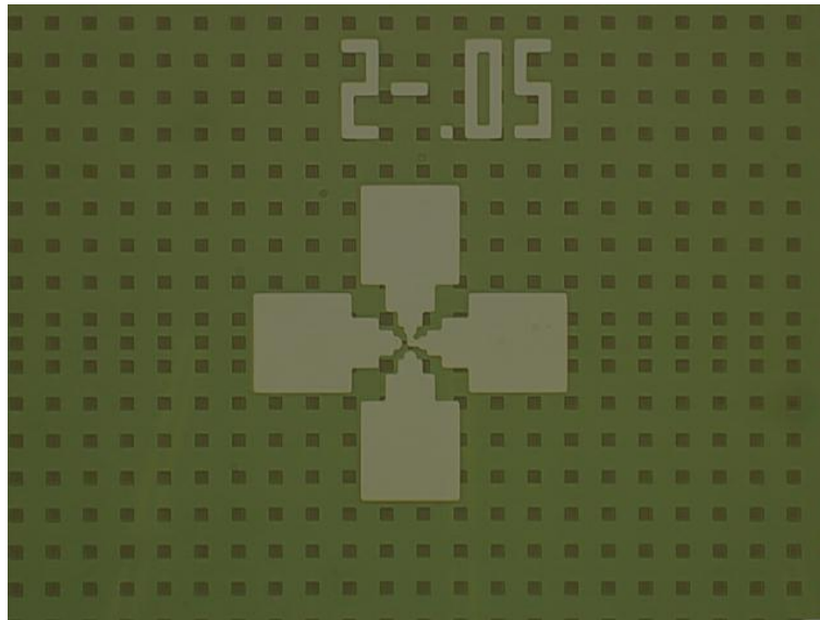
Fig. 3-3(e) OM image of the top view of the final CBKR structure. The magnification is 250x.
