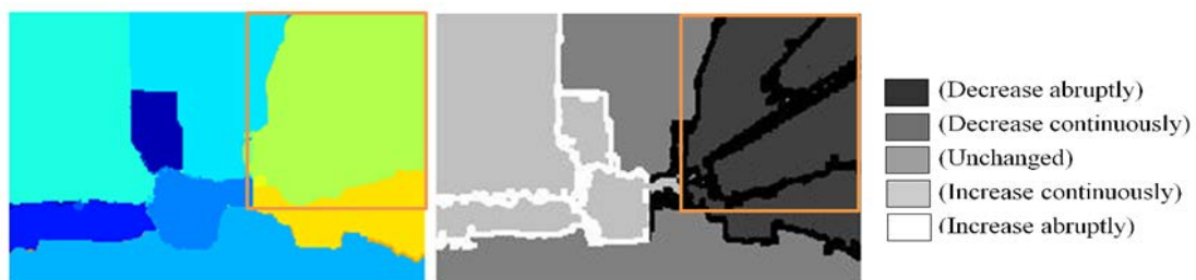
Figure 3-23 Example of how region consistency works to remove non-occlusion boundary. (a) Segmentation map. (b) Initial depth gradient map in the horizontal direction.
