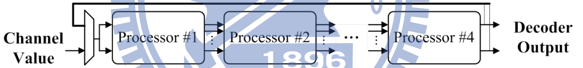
Figure 3.1: The illustration of a tail-biting LDPC convolutional code decoder.
