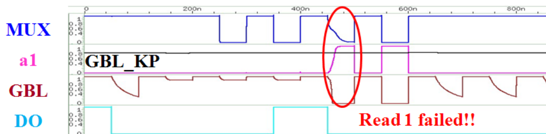
Fig. 3.24 The waveform for GBL by replica keeper @ ff, 125°C, VDD=1.1V.
