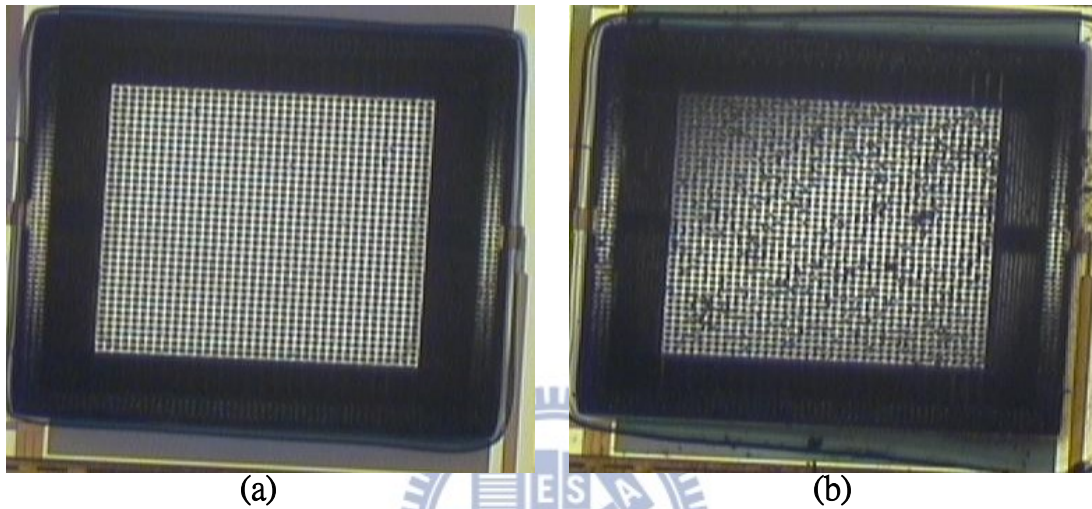
Figure 2.15: The OM Photos of the accelerometer from T18-101B: (a) the part of proof mass with more reflection, and (b) the part of proof mass with less reflection
