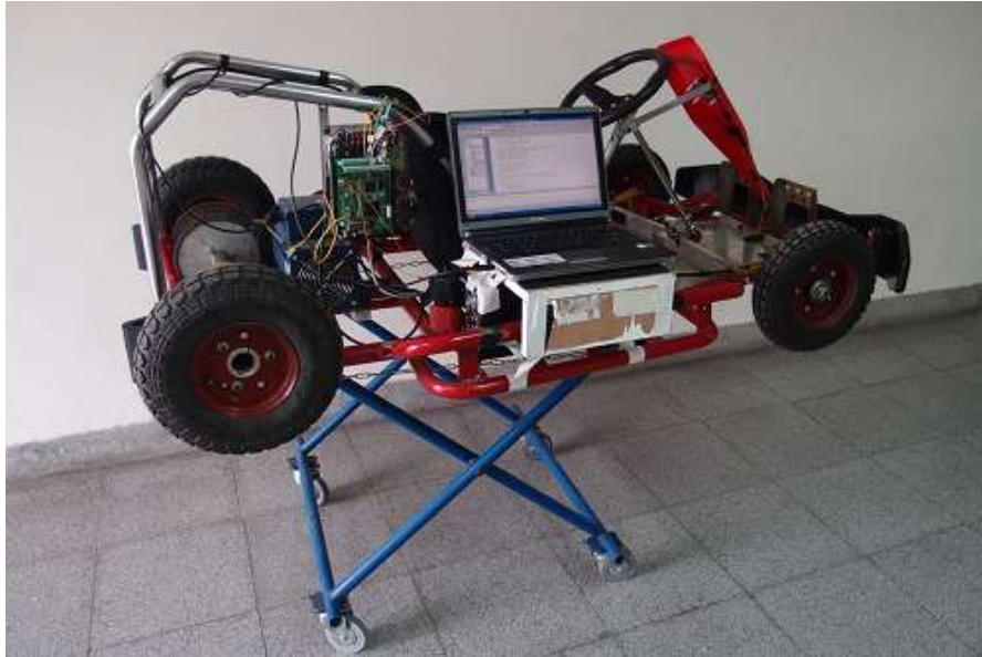
Fig. 3-6 Experimental setup of rotor time constant identification performed directly on the vehicle
