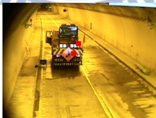
Fig. 3-15 False detection of flashing lights
