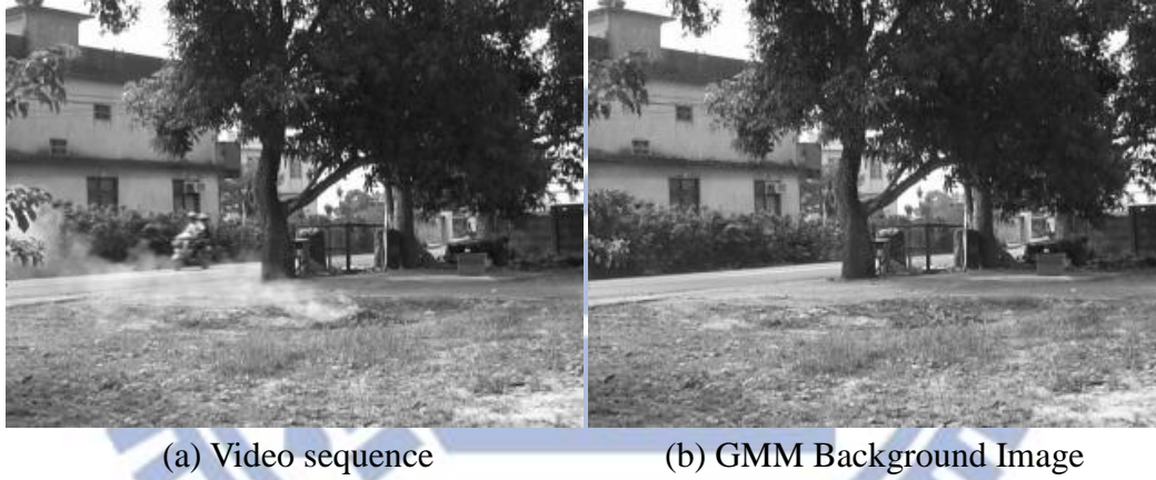
Fig. 3-3 Background image construction by GMM
