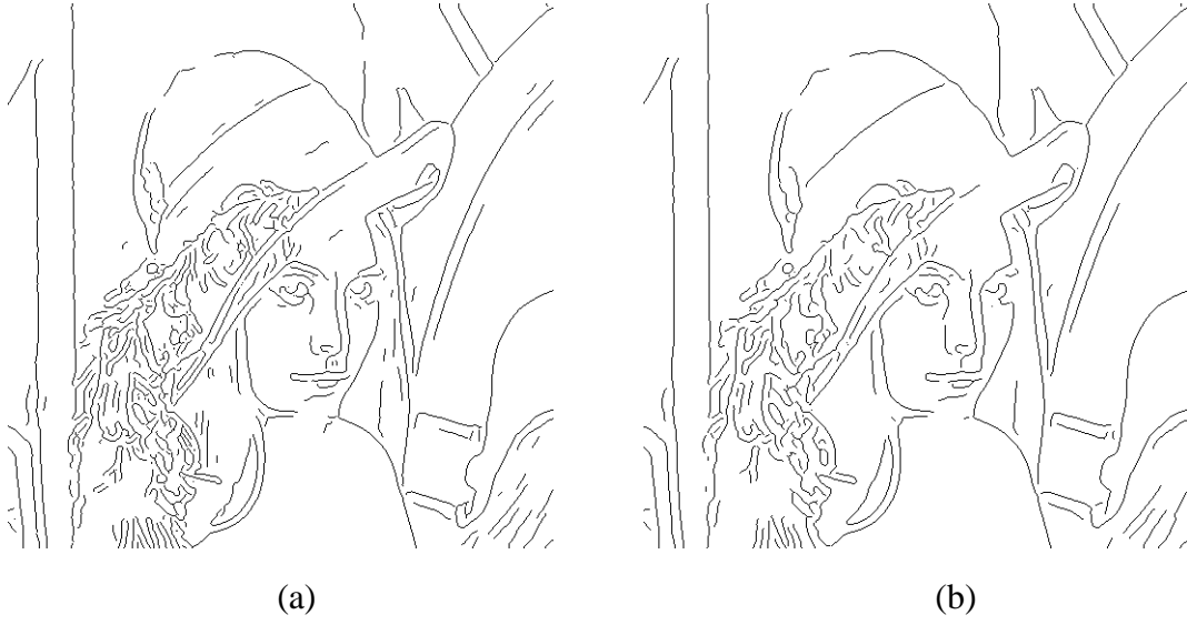
Fig.4.12 The results of Canny edge detector[11] for natural image “Lenna”, (a) \sigma = 1.6 , T_{Low} = 0.1 , T_{High} = 0.12 ; (b) \sigma = 2 , T_{Low} = 0.1 , T_{High} = 0.12 .
