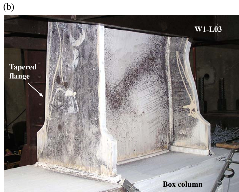
Figure 4.9 Plastic hinge formation followed by local buckling at 5% rad story drift angle: (a) specimen W1-L05; (b) specimen W1-L03.
