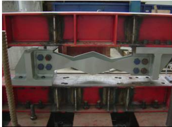
(a) 試體 FS12T (切削斷面, \beta = 0.33 )
