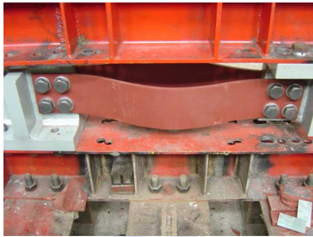
(b) 試體 FS12U (均勻斷面, \beta = 1.0 )
