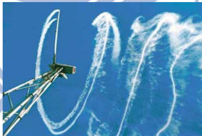
Fig. 1.4 Wake effect from wind turbine picture (Riso National Laboratory, Denmark) [20]
