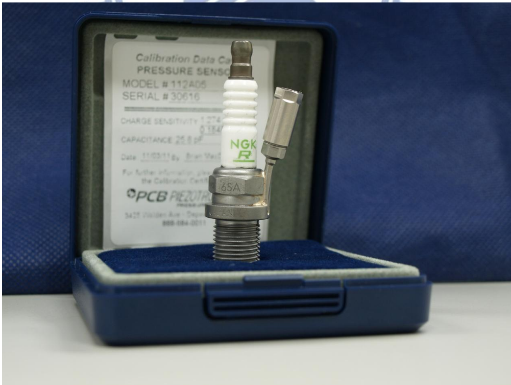
Figure 3.13 Spark Plug Pressure Sensor (BKR5E-11 and 112A05)
