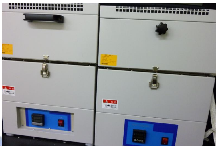
Figure 3.7: The furnaces for heating system
