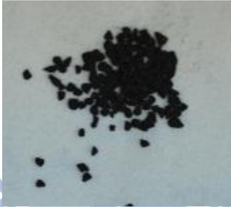
Figure Appendix C. 3: 10 wt % \text{Ni}_{0.35}\text{Mg}_{2.65}\text{FeO}_{4.5}/\text{Al}_2\text{O}_3 after hydrogen reduction through 5-0.5 hr at the hydrogen flow rates of 50-30 sccm.
