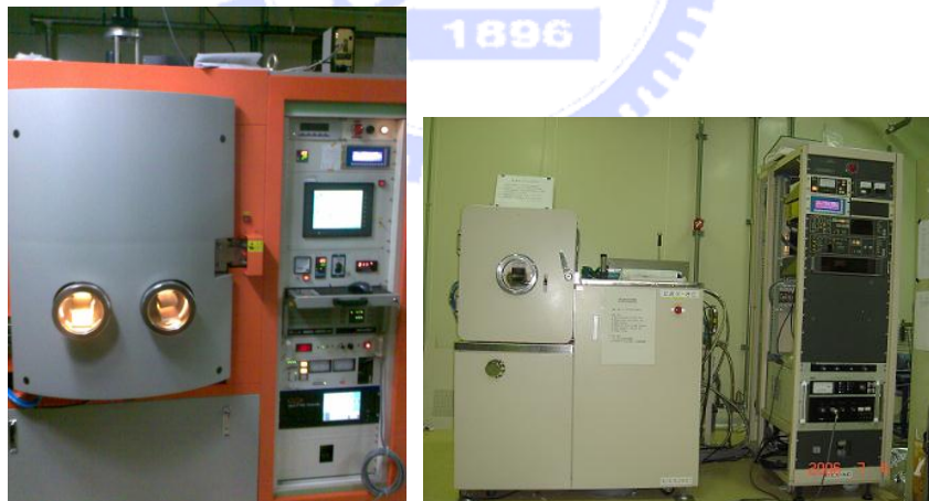
Fig. 2.7 Coating system with optical in-situ monitor (KS-800OPTO) and E-gun evaporator (ULVAC EBX-8C)
