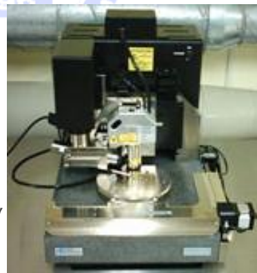
Fig. 2.15 The AFM feedback loop. A compensation network monitors the cantilever deflection and keeps it constant by adjusting the height of the sample. Atomic Force Microscope (D3100)
