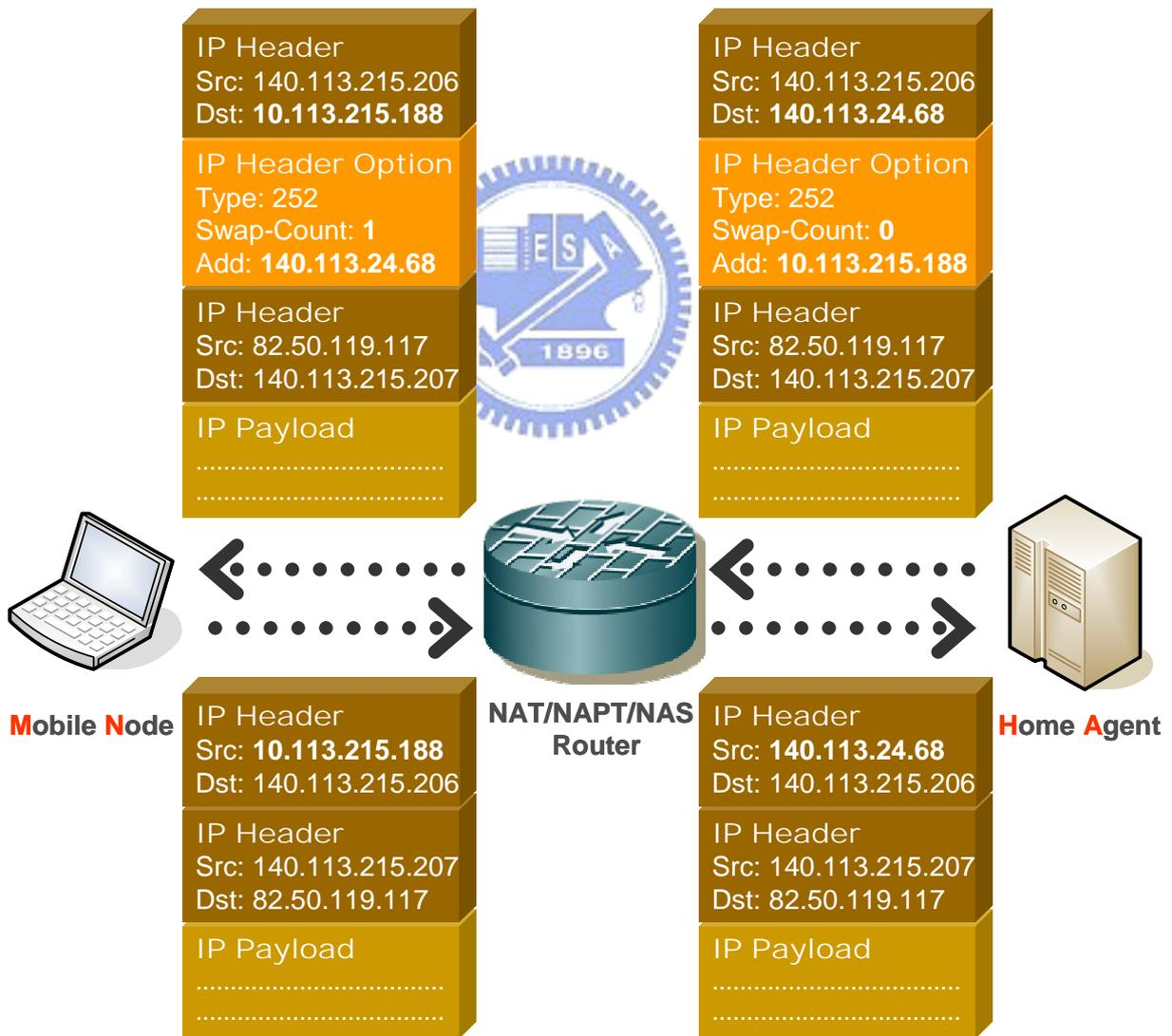
Figure 5 - 8: IP-in-IP<sup>HO</sup> Tunneling and IP-in-IP Reverse Tunneling
