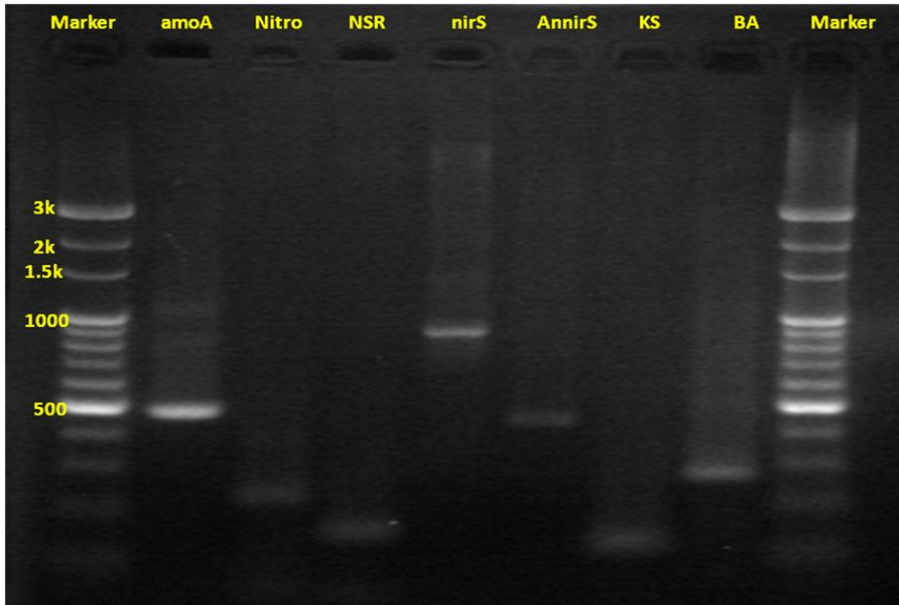
Figure 18 Results of PCR by performing agarose gel electrophoreses. The sample was taken on day 229 from SBR-18.
