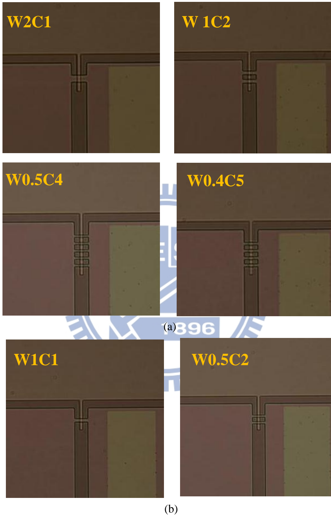
Fig. 3-2 The top view optical microscope microphotograph of MILC-VTFTs with various widths of crystal filter. (a) Total width = 2 \mu\text{m} (b) Total width = 1 \mu\text{m}
