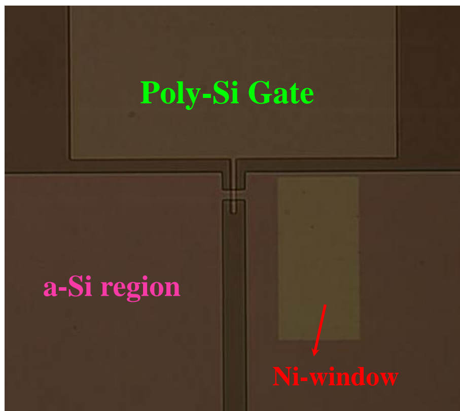
Fig. 2-7 Optical microscopy photograph of active pattern with the source, the drain, channels, bottom-gate and Ni-seeding window.
