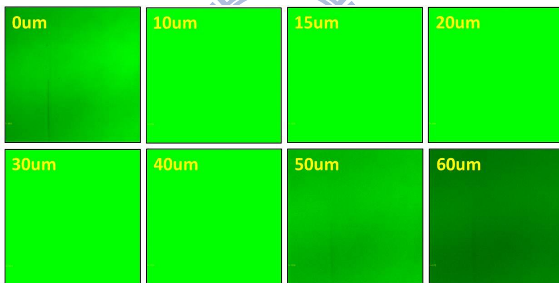
Fig. 4-5 The fluorescent light intensity of each LC layers with no driven voltage.
