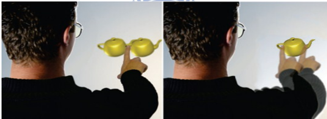
Fig. 17. Main issue in 2D touch interface with stereoscopic data is that a user is either focus on the finger or the 3D virtual objects which both degrades the visual perception. [18]
