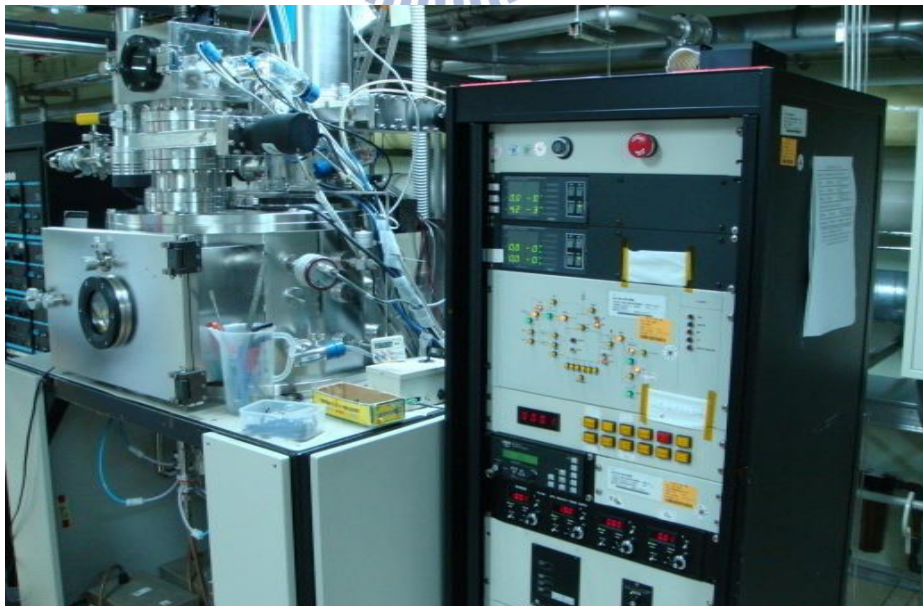
Fig. 3-2 The Sputtering system in NCTU.
