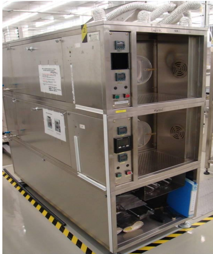
Fig. 3-3 Atmospheric anneal furnace.
