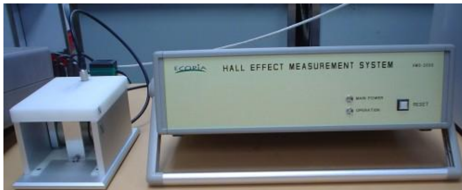
Fig. 3-7 Hall Effect Measurement System in NCTU.
