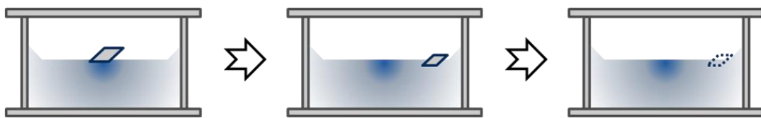
Fig. 5.4 Schematic drawing of dissolution of formed crystal in unsaturated region. Deep blue means the high concentration area induced by trapping laser.
