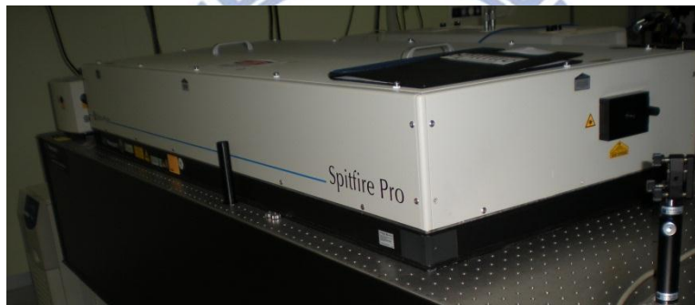
Fig.2.5 A picture of Ti:sapphire regenerative amplifier system, Spitfire
