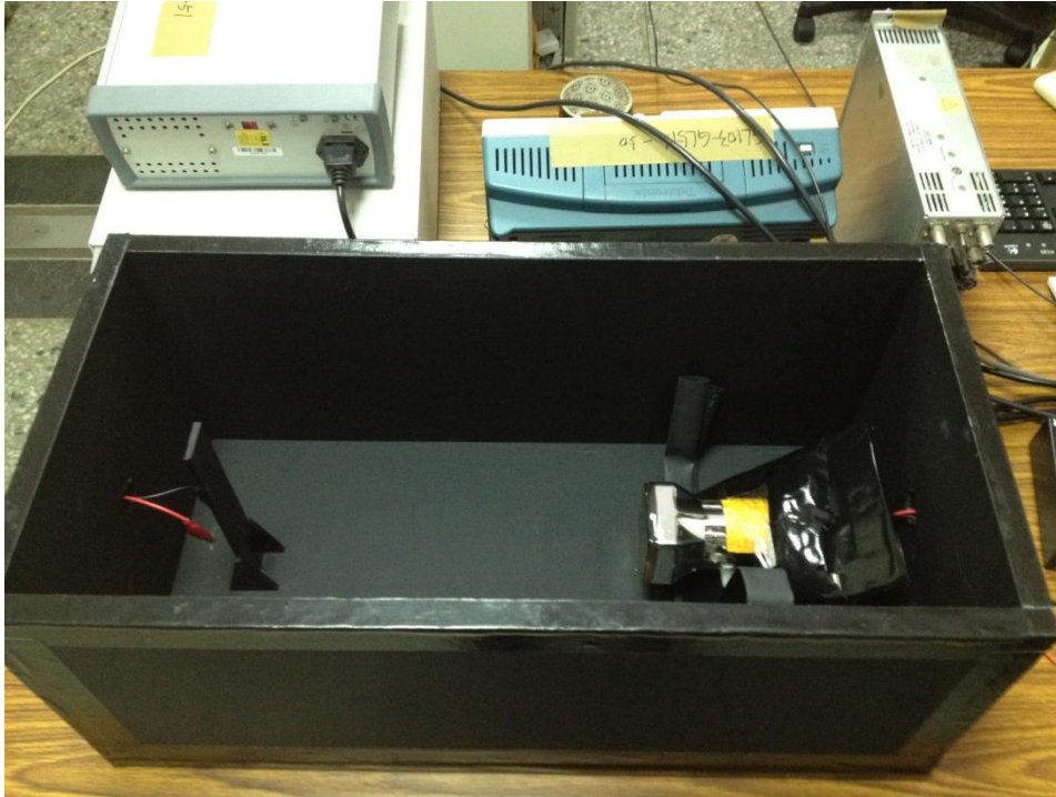
Fig. 3.9: The PMT was placed on the right side, LED was attached to the black stick on the left side.
