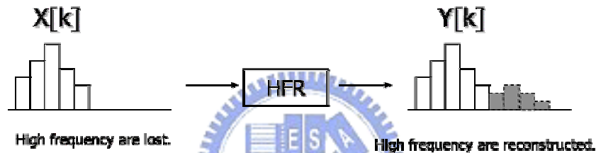
Figure 4: Block diagram of high frequency reconstruction.
