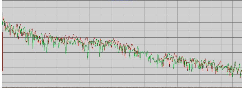
Figure 31: The unsuitable spectrum in Figure 30 is adjusted after envelope adjustment module.
