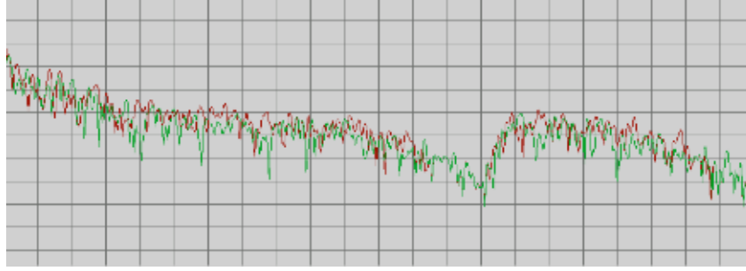
Figure 30: A spectrum with an unsuitable envelope on high frequency after spectrum duplication module.
