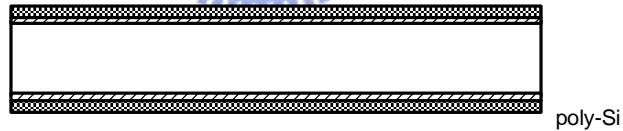
(c) deposition of LPCVD poly-Si
