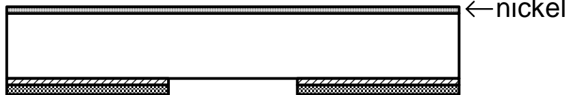
(f) Ni sputtering and annealing
